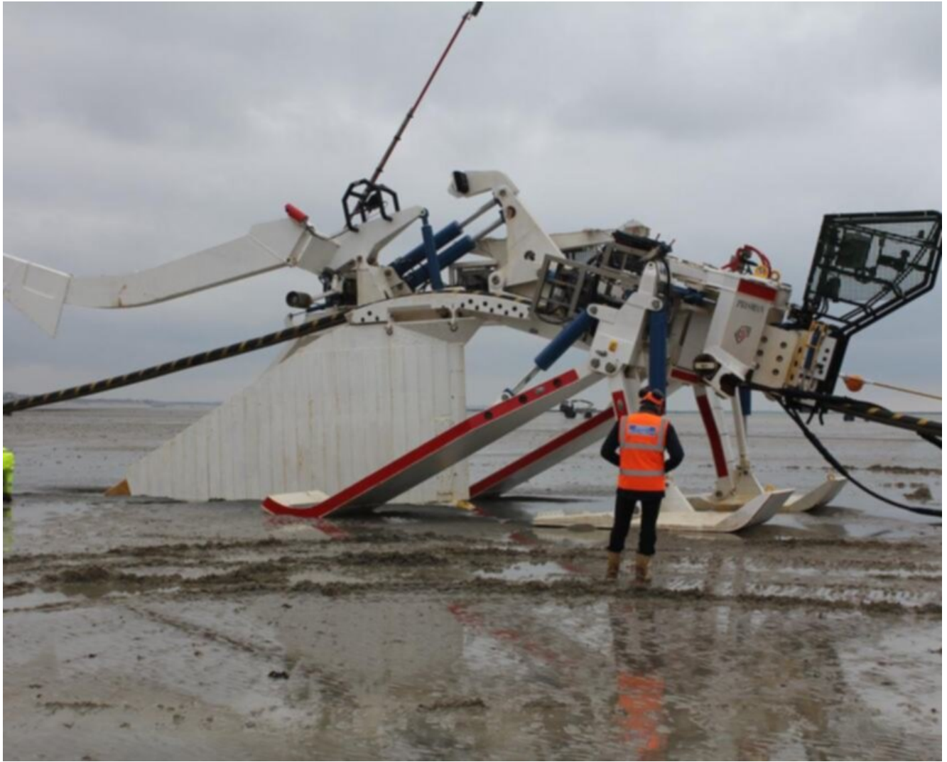
Prysmian's HD Power Cable plough (built by Soil Machine Dynamics) on Normandy Beach
